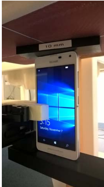
Photo of the device positioned for WR mode measurement – top edge facing phantom. The spacer was removed before the start of the measurements.
