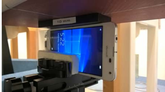
Photo of the device positioned for WR mode measurement – left edge facing phantom. The spacer was removed before the start of the measurements.
