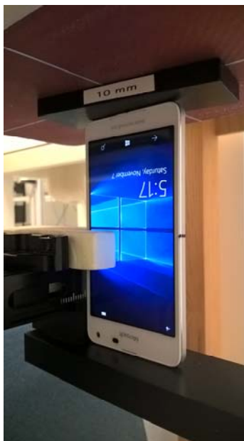
Photo of the device positioned for WR mode measurement – bottom edge facing phantom. The spacer was removed before the start of the measurements.
