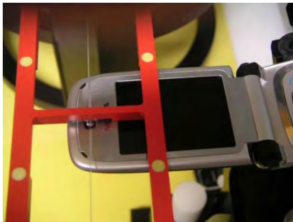
Photo of the device positioned under Test Arch and coordinate system (The EUT in picture is generic phone sample and does not represent the actual equipment under test)
