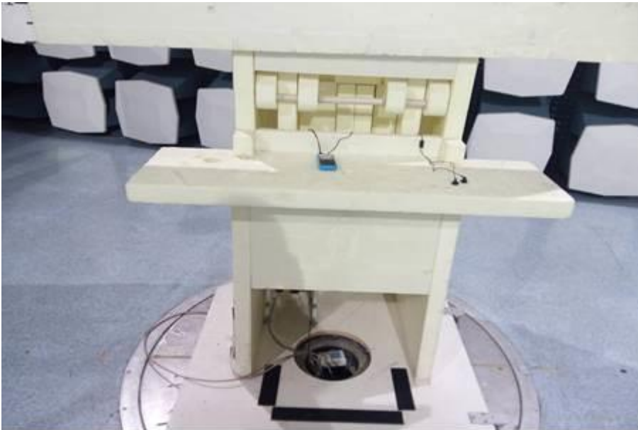
Picture 1. FCC Part 15B Radiated emissions
