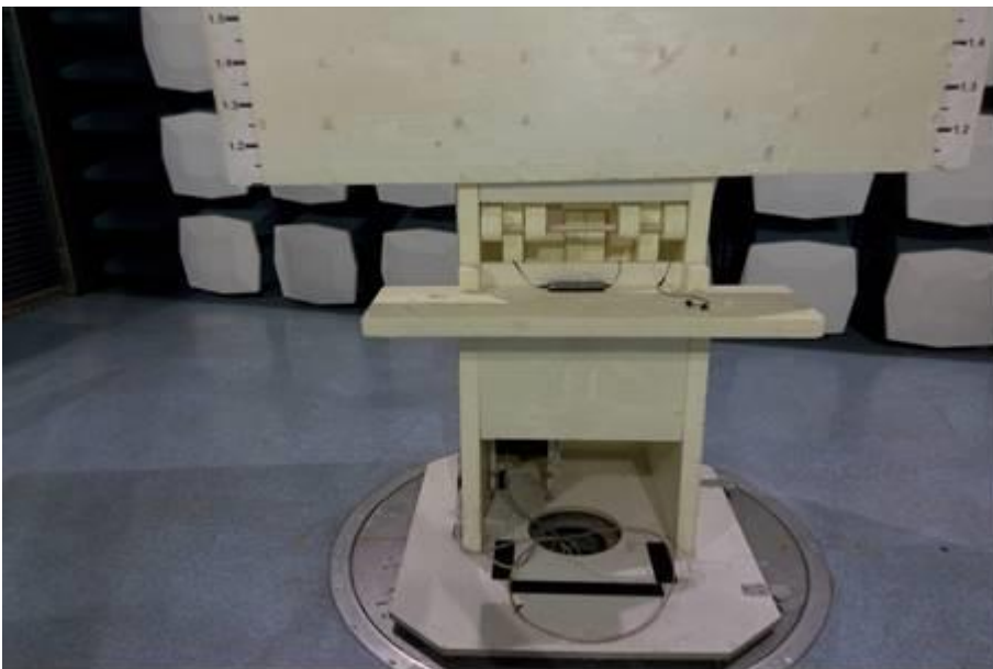
Picture 2. FCC Part 15B Radiated emissions
