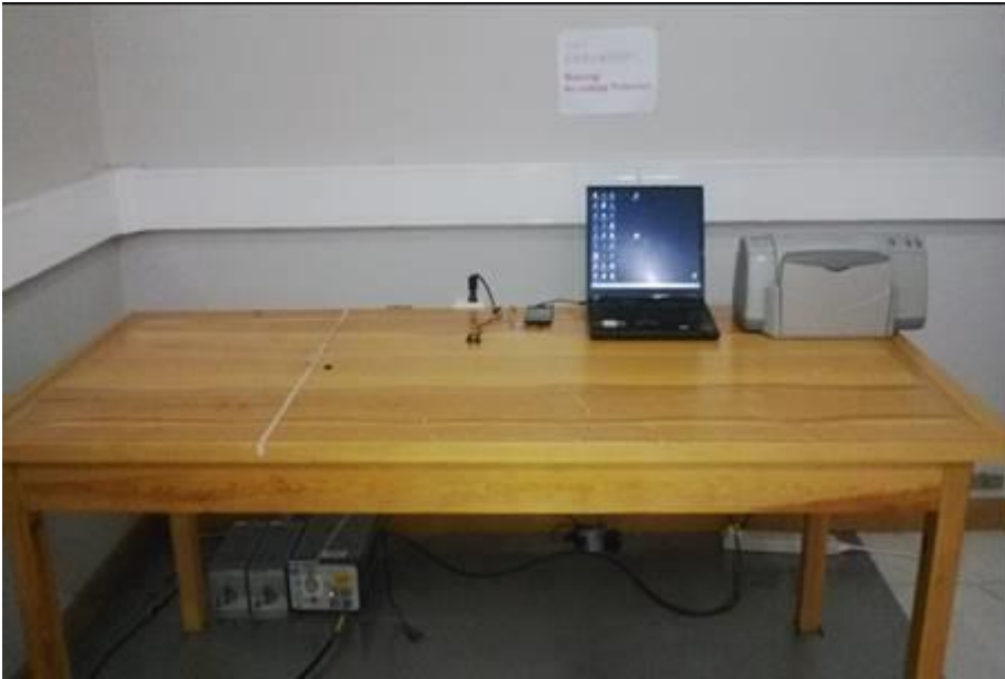
Picture 5. FCC Part 15B AC powerline conducted emissions, computer peripherals, measure from PC charger
