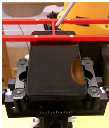
Photo of the device positioned under Test Arch
