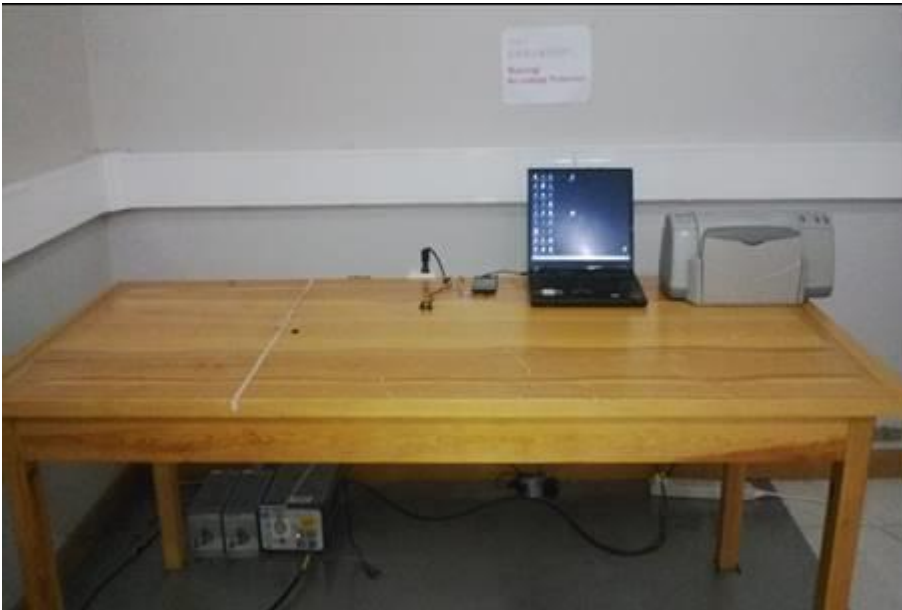
Picture 3. FCC Part 15B AC powerline conducted emissions, computer peripherals, measure from PC charger
