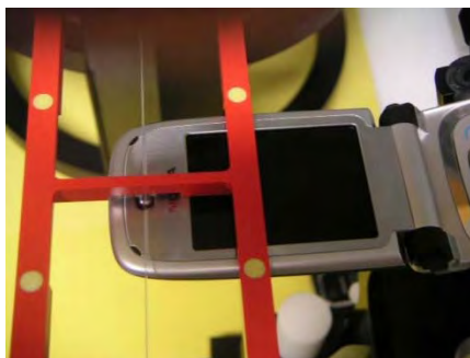
Photo of the device positioned under Test Arch and coordinate system (The EUT in picture is generic phone sample and does not represent the actual equipment under test)
