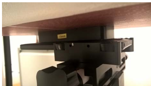
Photo of the device positioned for Body SAR measurement. The spacer was removed for the tests.
