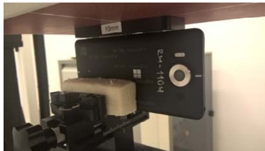
Photo of the device positioned for WR mode measurement – right edge facing phantom. The spacer was removed before the start of the measurements
