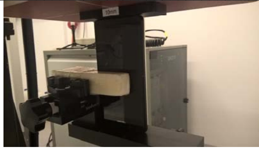
Photo of the device positioned for WR mode measurement – bottom edge facing phantom. The spacer was removed before the start of the measurements.
