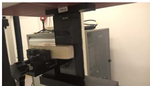
Photo of the device positioned for WR mode measurement – top edge facing phantom. The spacer was removed before the start of the measurements.
