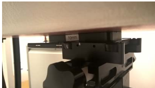
Photo of the device positioned for WR mode measurement – display facing phantom. The spacer was removed before the start of the measurements.
