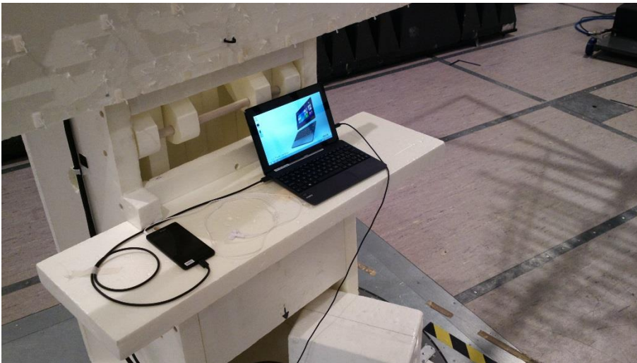
Picture 2. FCC Part 15B Radiated emissions
