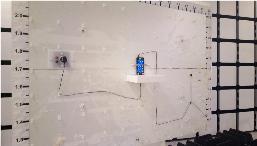
Picture 1. FCC Part 15C Radiated emissions
