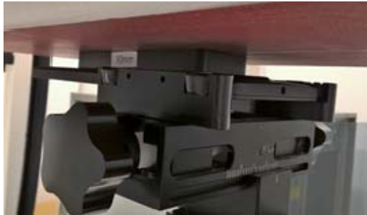
Photo of the device positioned for WR mode measurement –back facing phantom. The spacer was removed before the start of the measurements.
