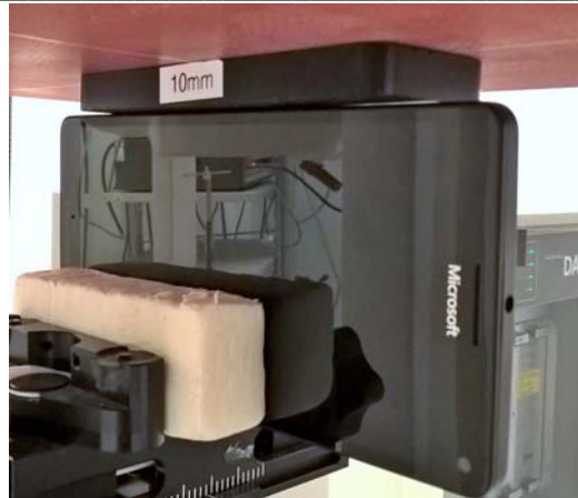
Photo of the device positioned for WR mode measurement – left edge facing phantom. The spacer was removed before the start of the measurements.
