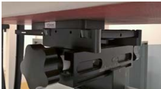
Photo of the device positioned for WR mode measurement – display facing phantom. The spacer was removed before the start of the measurements.
