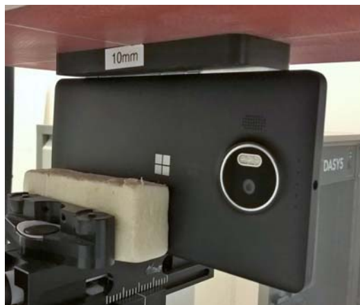
Photo of the device positioned for WR mode measurement – right edge facing phantom. The spacer was removed before the start of the measurements
