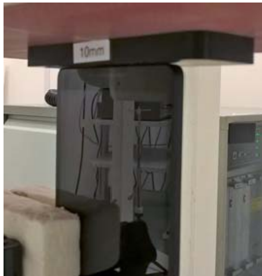
Photo of the device positioned for WR mode measurement – bottom edge facing phantom. The spacer was removed before the start of the measurements.
