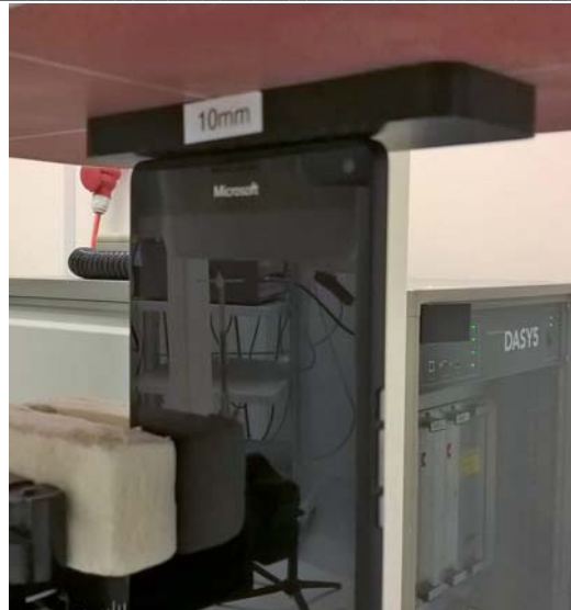
Photo of the device positioned for WR mode measurement – top edge facing phantom. The spacer was removed before the start of the measurements.
