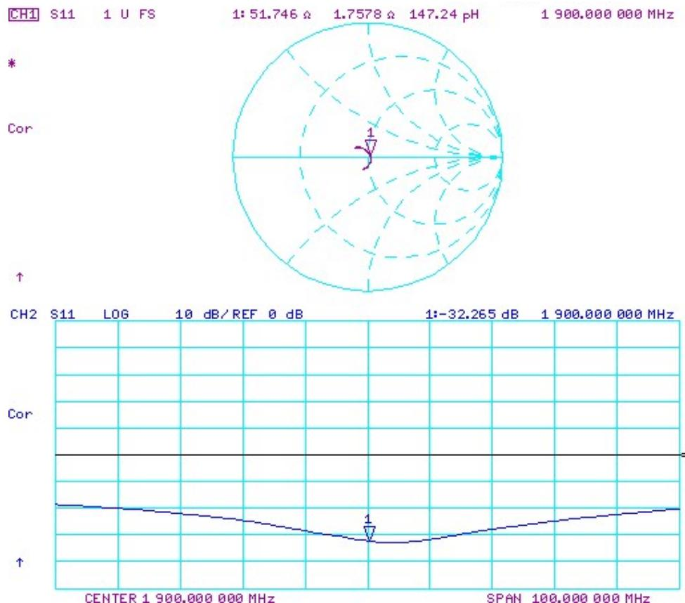
**Antenna Parameters with Body TSL**
