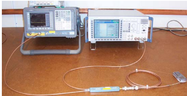
Picture 3: Test setup for conducted measurements
