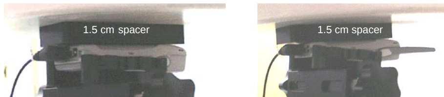
Photos of the device positioned for Body SAR measurement with flip closed and open. The spacer was removed for the tests.
