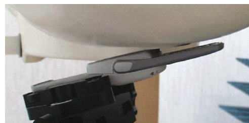
Photo of the device with flip open in “tilt” position.
