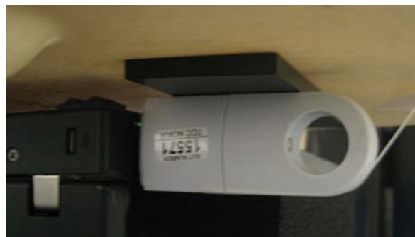
Device directly connected to a vertical USB port of the Lenovo laptop computer, side 3 facing the phantom. The 0.5 cm spacer was removed before the test.
