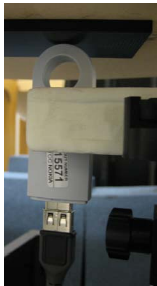
Device positioned below the phantom using a SPEAG device holder and expanded styrofoam blocks, side 5 facing the phantom. Device is connected to a USB port of the laptop computer using a CA-175D cable. The 0.5 cm spacer was removed before the test.
