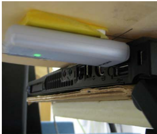
Device directly connected to a horizontal USB port of the IBM laptop computer, side 1 facing the phantom. The 0.5 cm spacer was removed before the test.
