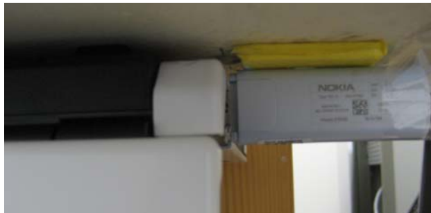
Device directly connected to a vertical USB port of the Amilo laptop computer, side 4 facing the phantom. The 0.5 cm spacer was removed before the test.
