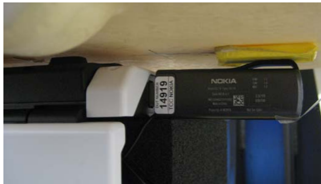
Device directly connected to a vertical USB port of the Amilo laptop computer, side 4 facing the phantom. The 0.5 cm spacer was removed before the test.
