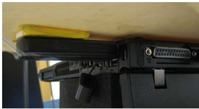
Device directly connected to a horizontal USB port of the IBM laptop computer, side 1 facing the phantom. The 0.5 cm spacer was removed before the test.
