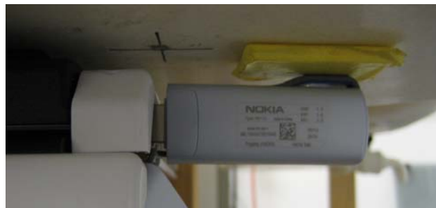
Device directly connected to a vertical USB port of the Amilo laptop computer, side 4 facing the phantom. The 0.5 cm spacer was removed before the test.
