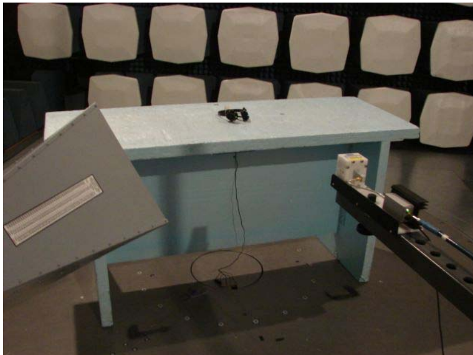
Picture 4: Radiated emission test setup 18 GHz – 25 GHz
