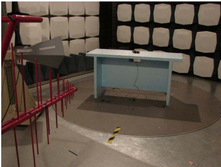
Picture 2: Radiated emission test setup &lt;1 GHz
