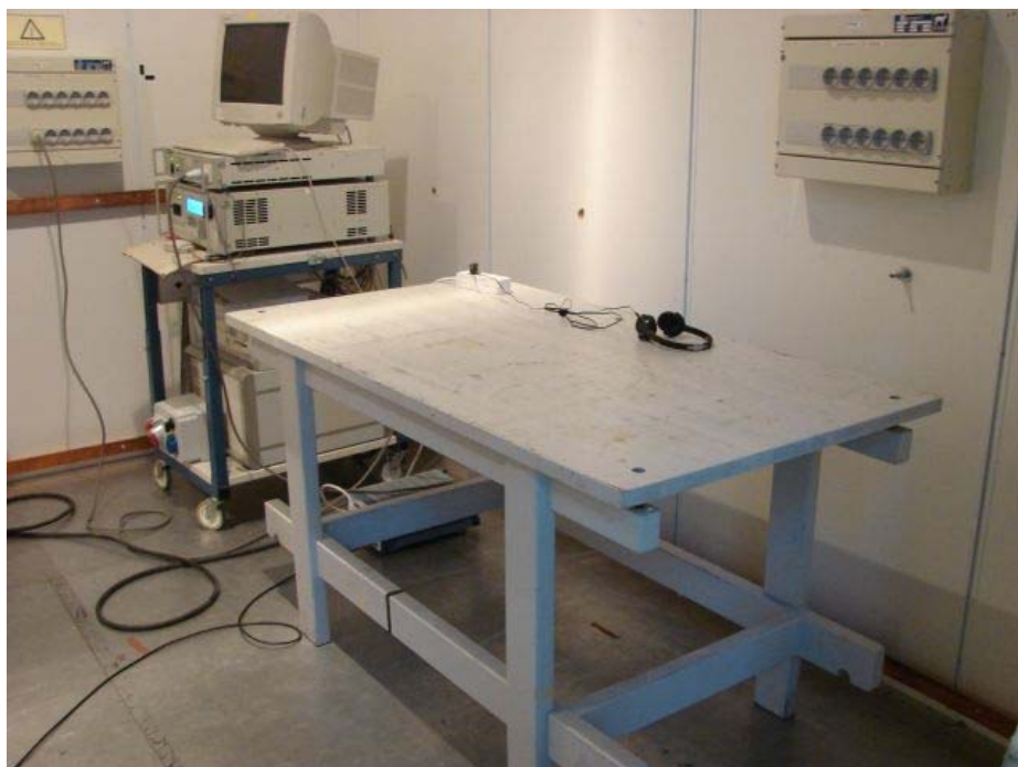
Picture 5: Conducted emissions to AC-mains test setup
