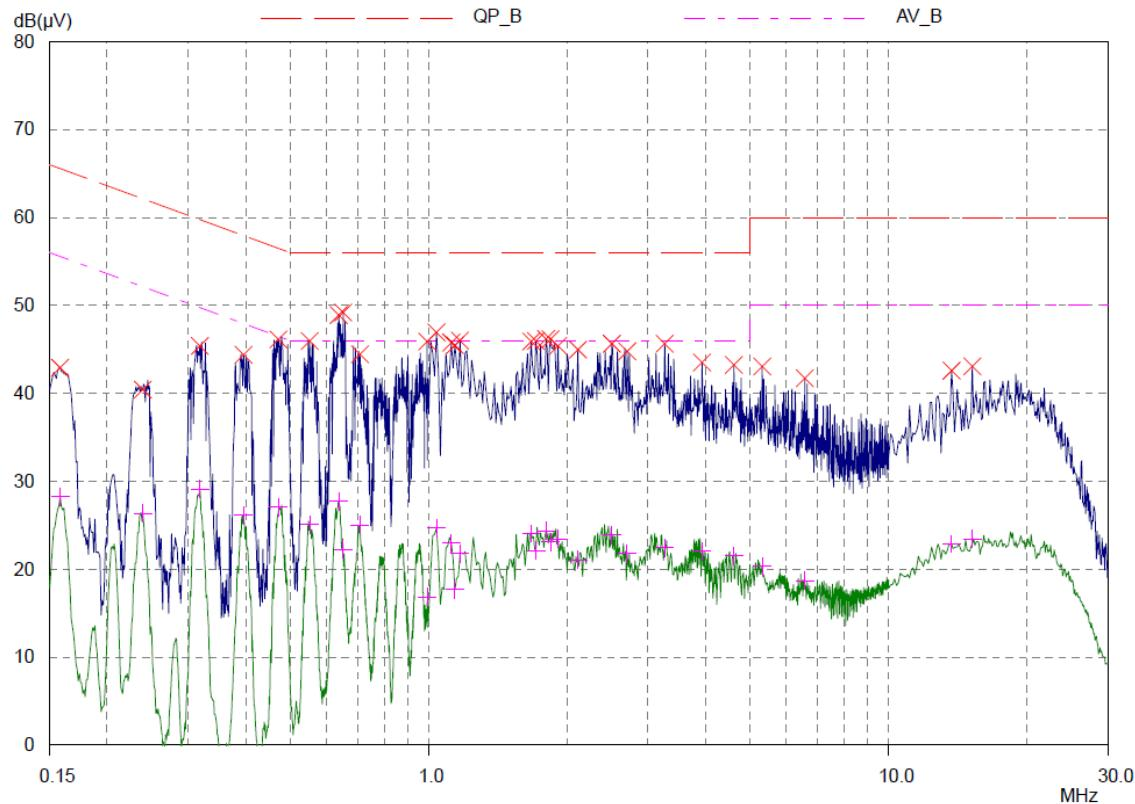
**ETL EMC Laboratory****Conducted Emission Test Result**
