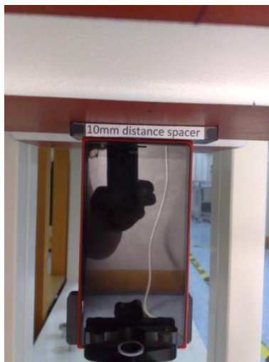
Photo of the device positioned for WR mode measurement – top edge facing phantom. The spacer was removed before the start of the measurements.
