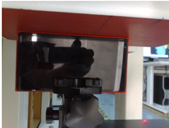
Photo of the device positioned for 10g Extremity measurement – left edge facing phantom.
