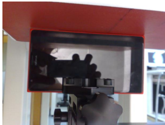
Photo of the device positioned for 10g Extremity measurement – right edge facing phantom.
