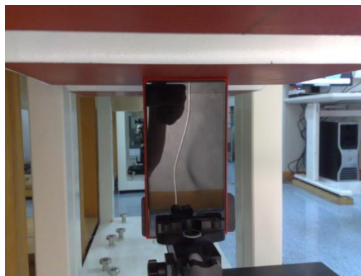
Photo of the device positioned for 10g Extremity measurement – bottom edge facing phantom.
