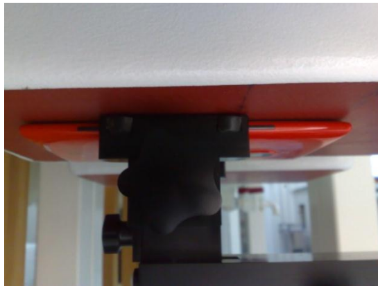
Photo of the device positioned for 10g Extremity measurement –display facing phantom.
