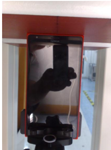
Photo of the device positioned for 10g Extremity measurement – top edge facing phantom.
