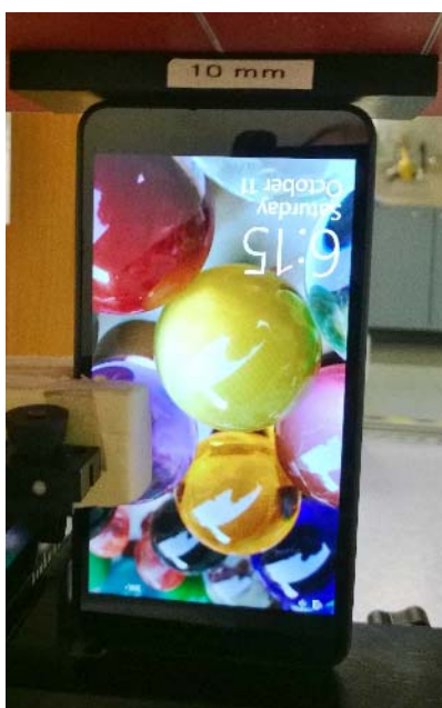
Photo of the device positioned for WR mode measurement – bottom edge facing phantom. The spacer was removed before the start of the measurements.
