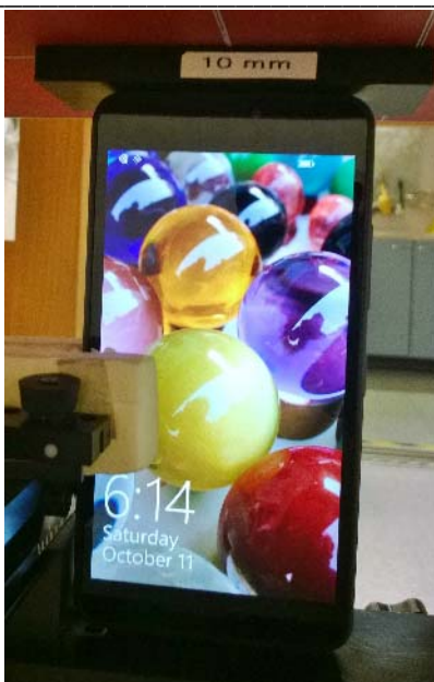
Photo of the device positioned for WR mode measurement – top edge facing phantom. The spacer was removed before the start of the measurements.
