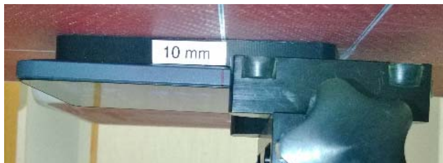
Photo of the device positioned for WR mode measurement –back facing phantom. The spacer was removed before the start of the measurements.
