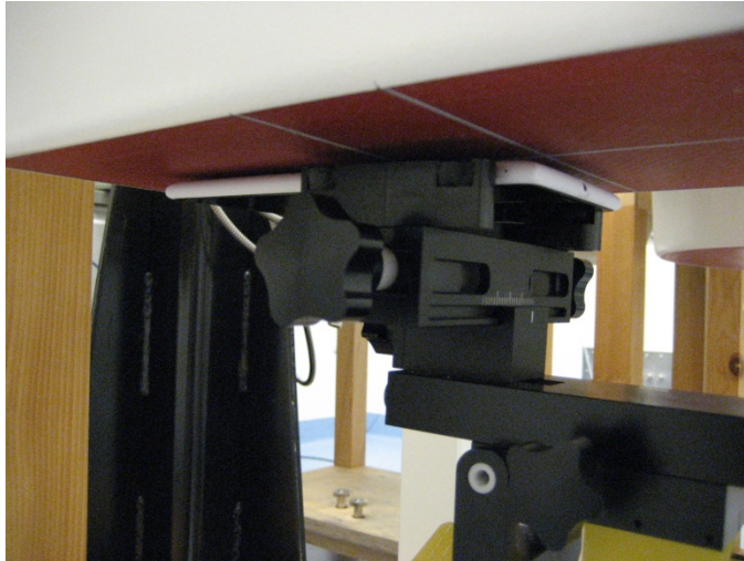
Photo of the device positioned for 10g Extremity measurement –back facing phantom.
