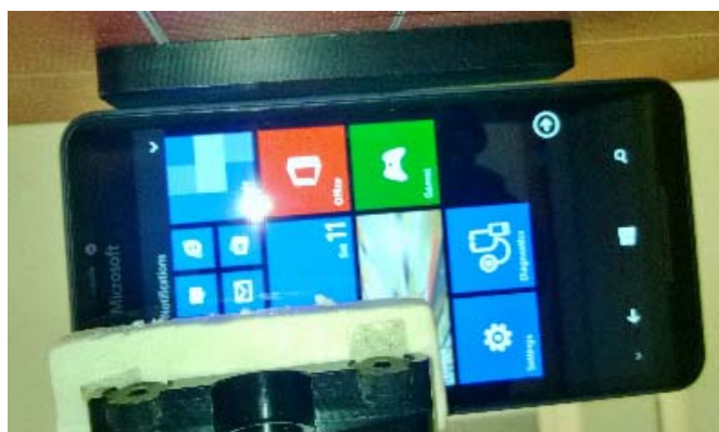
Photo of the device positioned for WR mode measurement – right edge facing phantom. The spacer was removed before the start of the measurements
