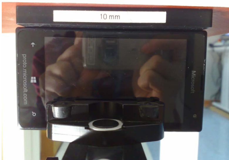
Photo of the device positioned for WR mode measurement – left edge facing phantom. The spacer was removed before the start of the measurements.
