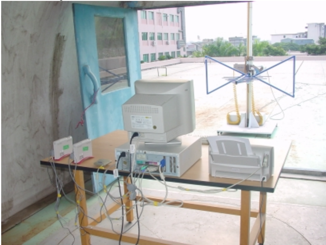
Photo 4 Test Setup for Radiated Test (Rear View)
