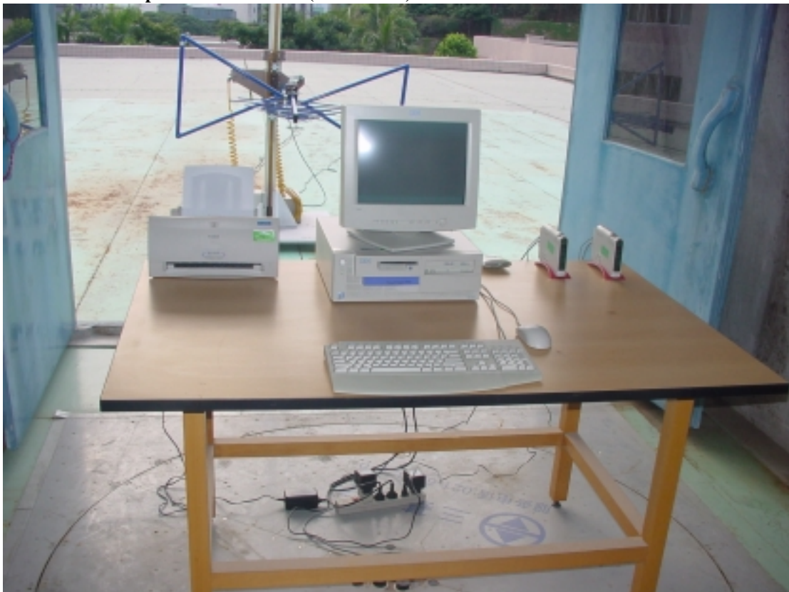
Photo 3 Test Setup for Radiated Test (Front View)
