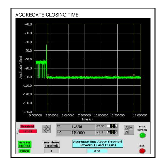
No transmissions are observed during the aggregate monitoring period.
