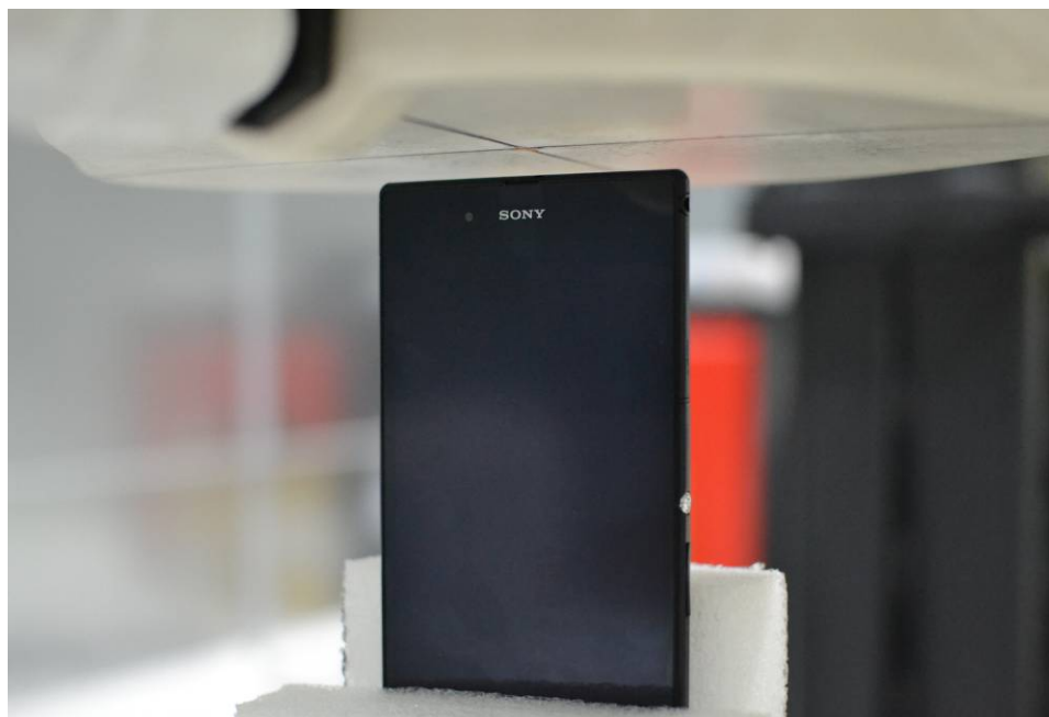
SAR Test Setup Photo 7 – Top Edge at 5 mm
