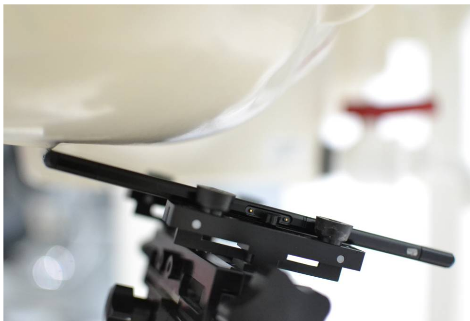
SAR Test Setup Photo 2 – Right Tilt
