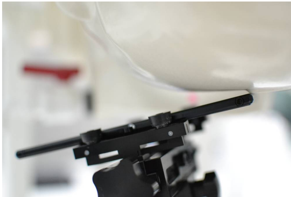
SAR Test Setup Photo 4 – Left Tilt
