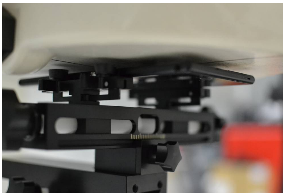
SAR Test Setup Photo 6 – Front side at 5 mm
