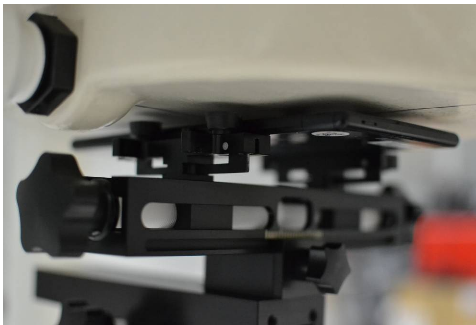
SAR Test Setup Photo 5 – Back side at 5 mm
