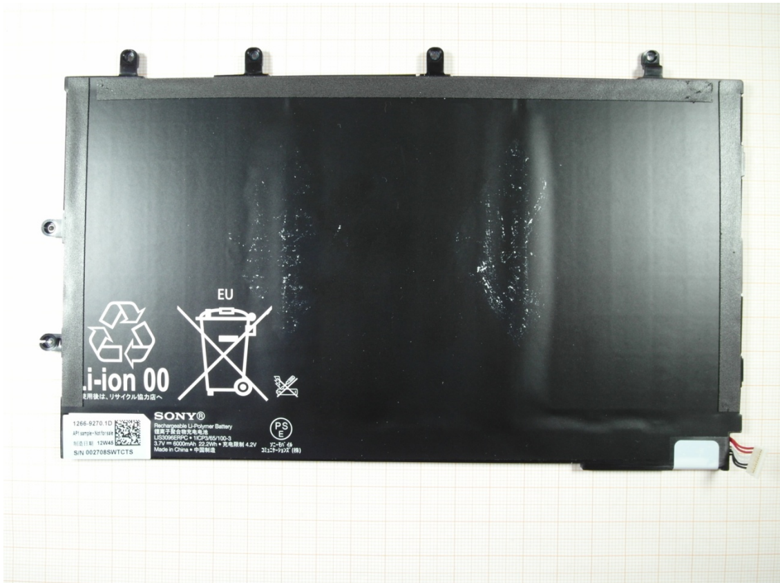
EUT inside, Battery (Li-Ion, front side)
