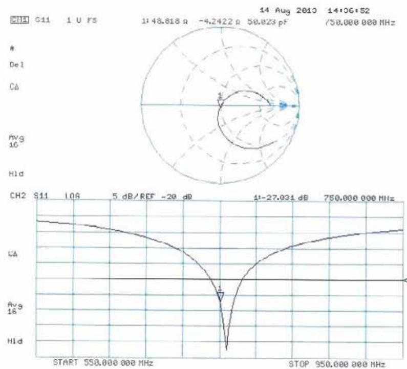
**5 Calibration report “835 MHz System validation dipole”**
