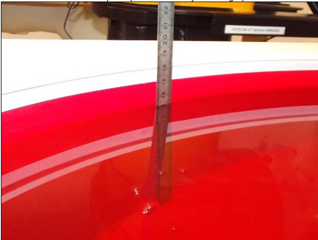
Photo 3: Liquid depth 1750 MHz body simulating liquid
