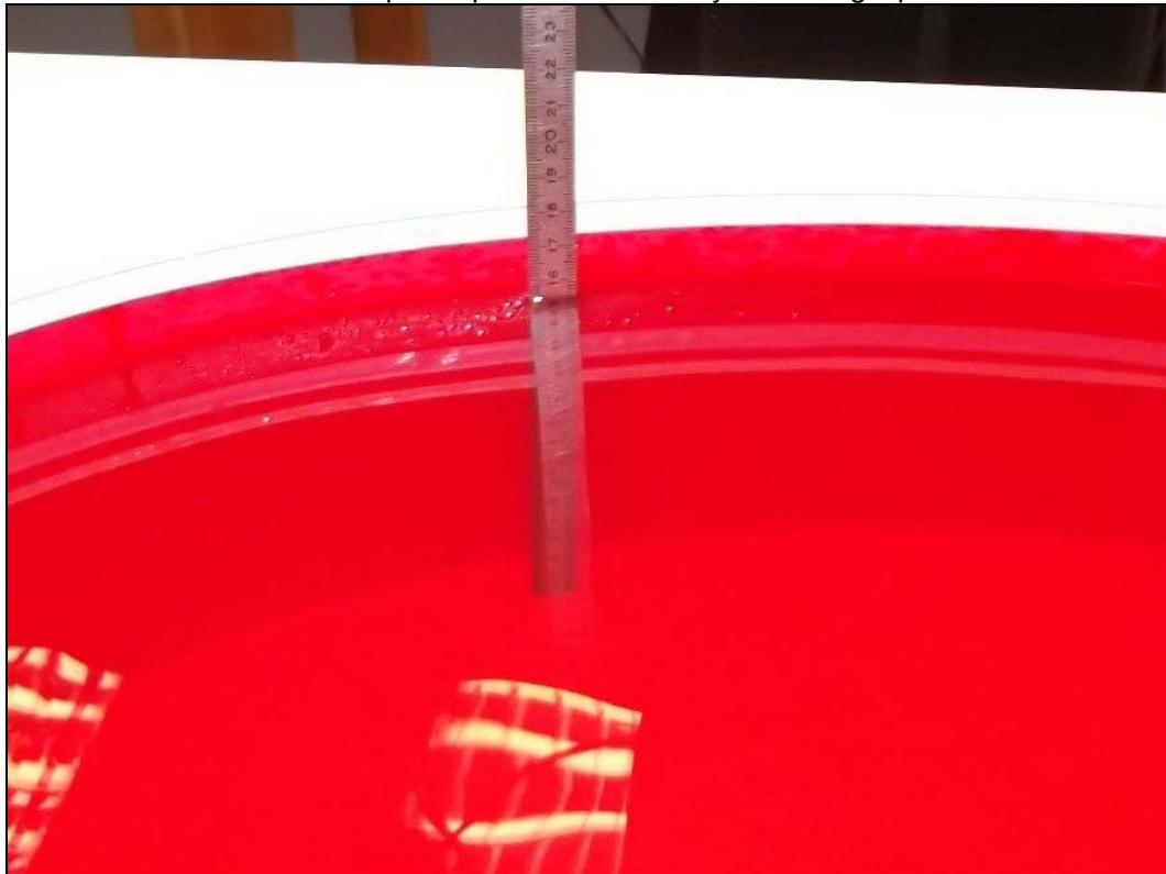
Photo 6: Liquid depth 5 GHz body simulating liquid
