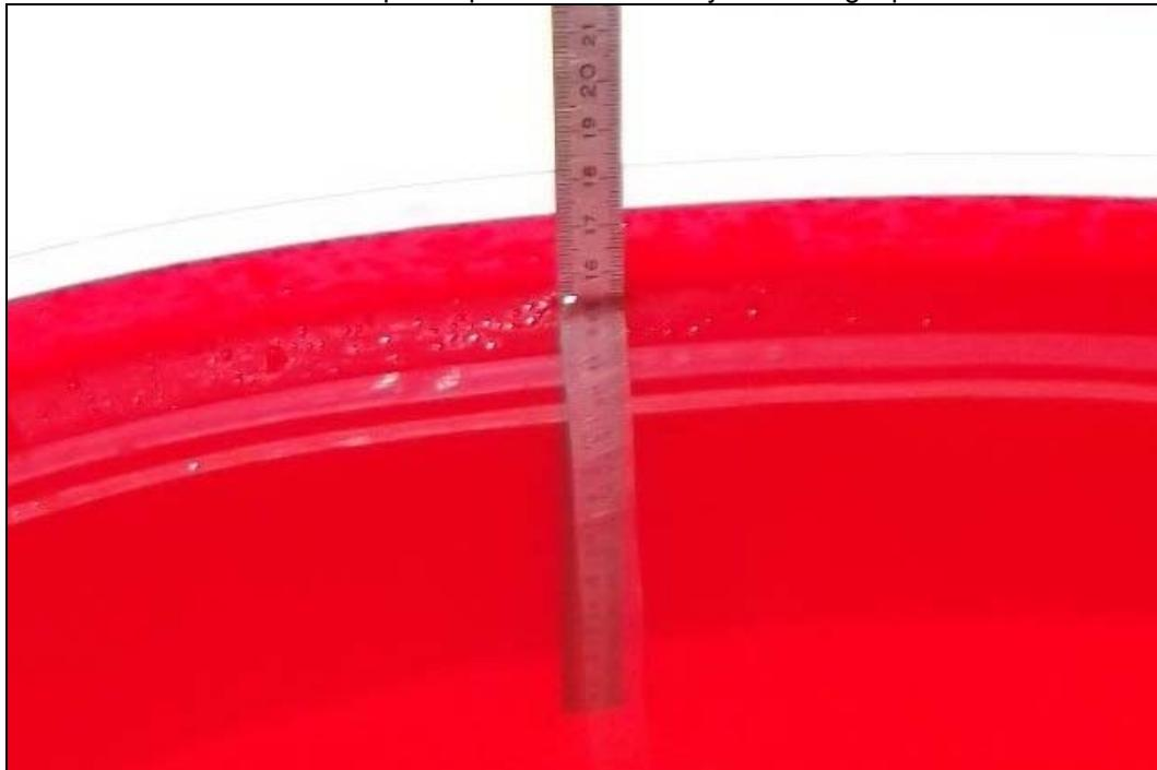
Photo 4: Liquid depth 1900 MHz body simulating liquid
