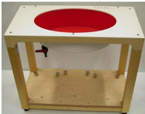
The ELI4 phantom is intended for compliance testing of handheld and body-mounted wireless devices in the frequency range of 30MHz to 6 GHz. ELI4 is fully compatible with the standard IEC 62209-2 and all known tissue simulating liquids.
