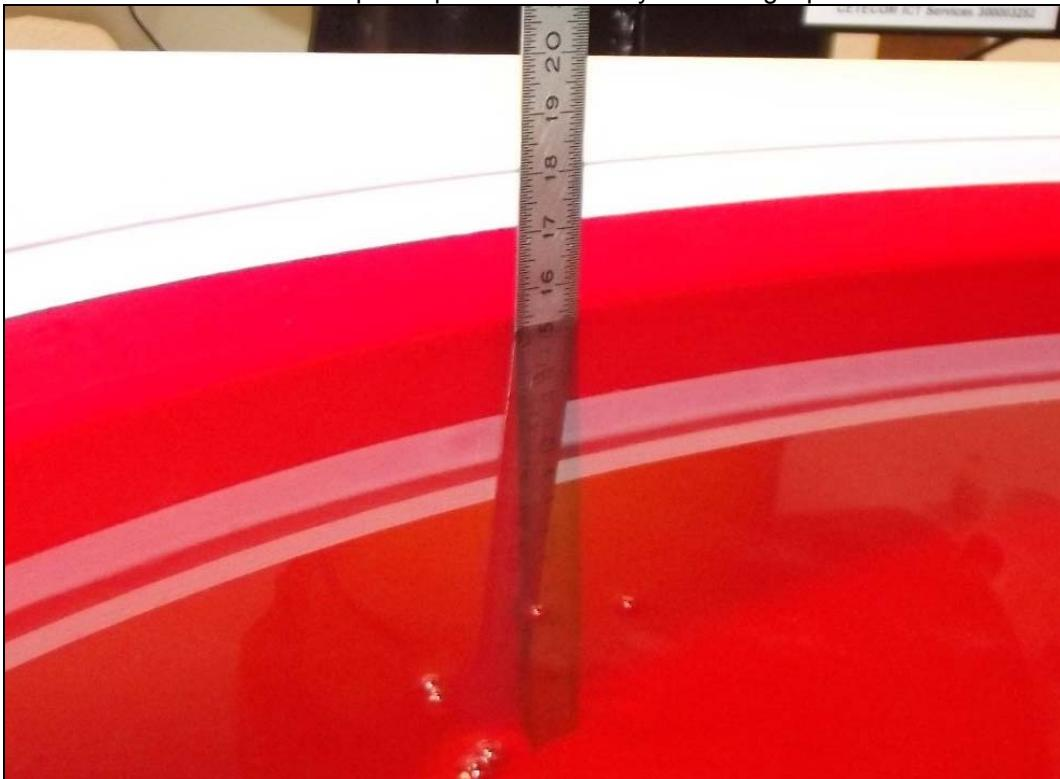
Photo 2: Liquid depth 850 MHz body simulating liquid
