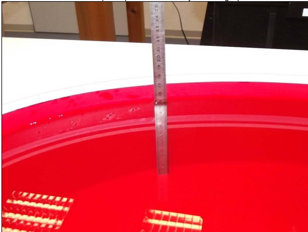
Photo 5: Liquid depth 2450 MHz body simulating liquid
