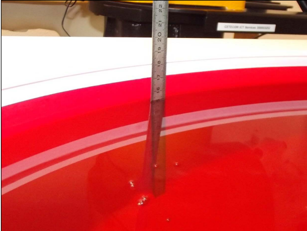
Photo 2: Liquid depth 1800 MHz body simulating liquid
