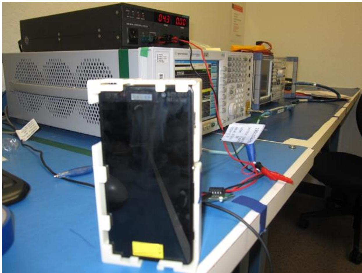
**RADIATED RF MEASUREMENT SETUP FOR PORTABLE CONFIGURATION**
