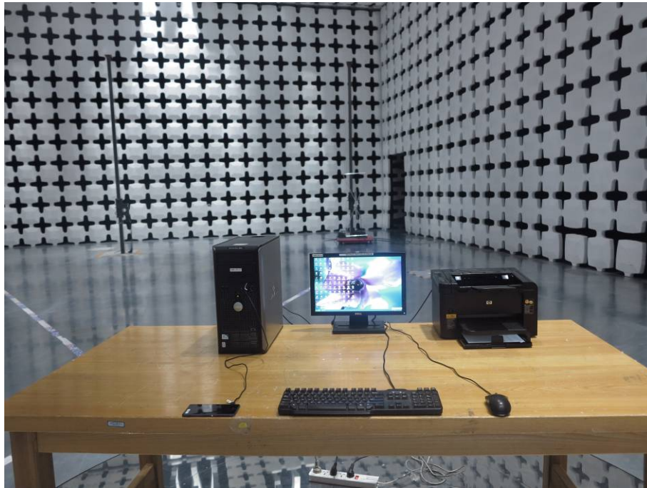
Picture C-7: Radiated emission (PART15B)
