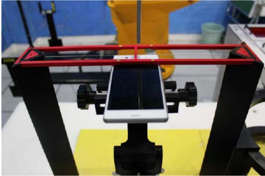
Picture C-11: EUT Positioning for T-coil(HAC)
