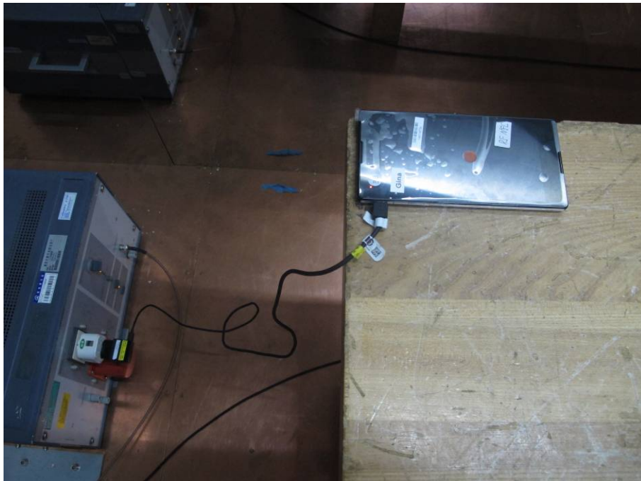
Picture C-14: AC Powerline Conducted Emission(PART15C)
