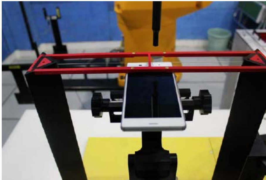
Picture C-10: EUT Positioning for RF(HAC)
