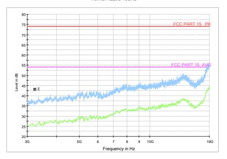
Fig.11. Radiated emission: Channel 78, 3 GHz - 18 GHz
