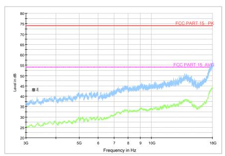
Fig.8. Radiated emission: Channel 39, 3 GHz - 18 GHz
