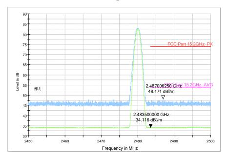
Fig.13. Radiated emission (Power): High Channel
