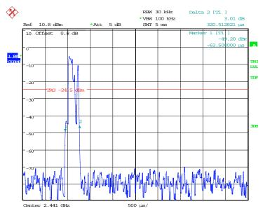
Fig.2. pulse width: Channel 39
