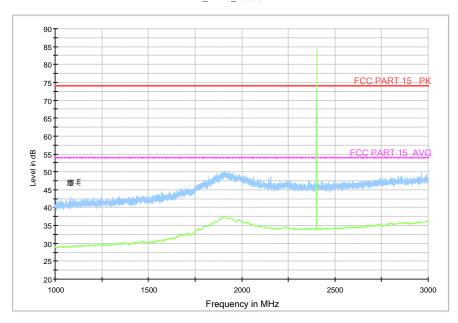
Fig.4. Radiated emission: Channel 0, 1 GHz - 3 GHz
