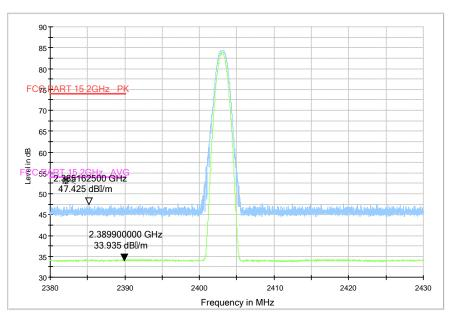
Fig.12. Radiated emission (Power): Low Channel
