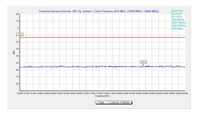
Fig.A.6.1.31 Conducted Spurious Emission (802.11g, Ch1, 15 GHz-20 GHz)
