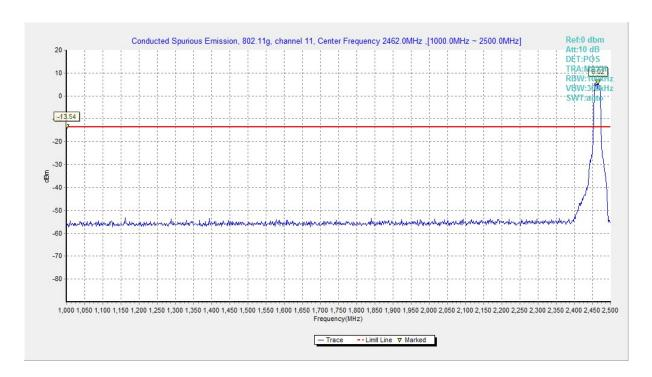
Fig.A.6.1.43 Conducted Spurious Emission (802.11g, Ch11, 1 GHz-2.5 GHz)
