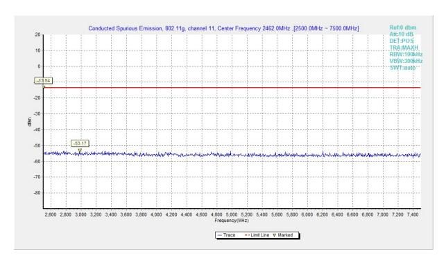
Fig.A.6.1.44 Conducted Spurious Emission (802.11g, Ch11, 2.5 GHz-7.5 GHz)
