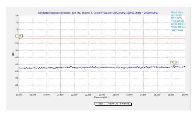
Fig.A.6.1.32 Conducted Spurious Emission (802.11g, Ch1, 20 GHz-26 GHz)
