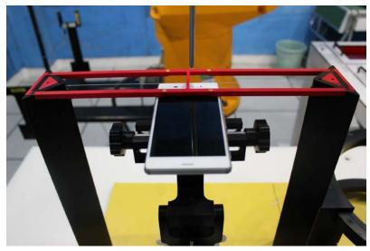
Picture 3: EUT Positioning for T-coil
