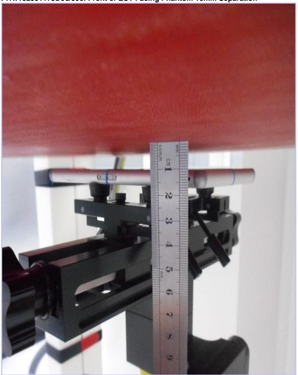
PHT/10295117JD06/007: Front of EUT Facing Phantom 15mm Separation
