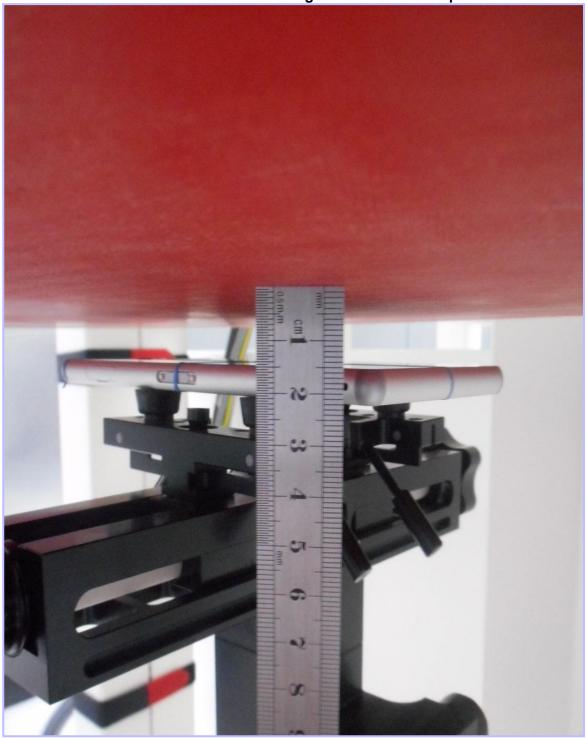
PHT/10295117JD06/008: Back of EUT Facing Phantom 10mm Separation
