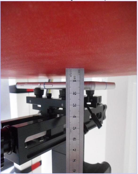
PHT/10295117JD06/009: Back of EUT Facing Phantom 15mm Separation
