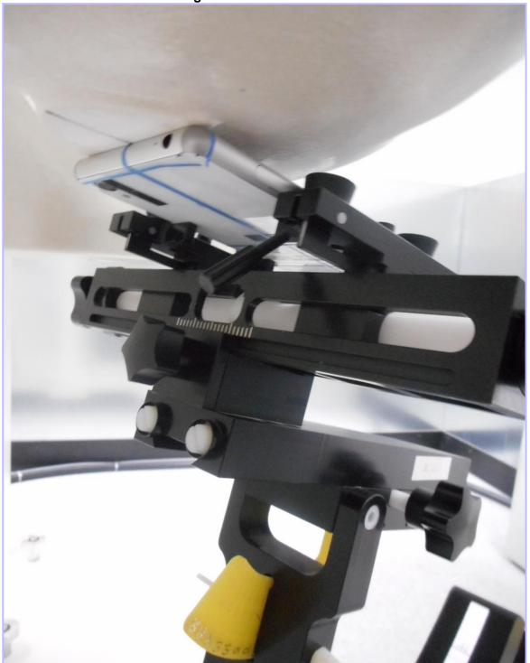
PHT/10295117JD06/006: Front of EUT Facing Phantom 10mm Separation
