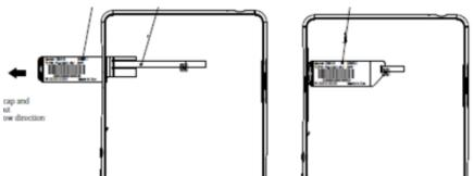
The FCC ID is not on the exterior of the device but labelling meets the conditions allowed in KDB 784748 for the label to be placed in a user accessible area:
