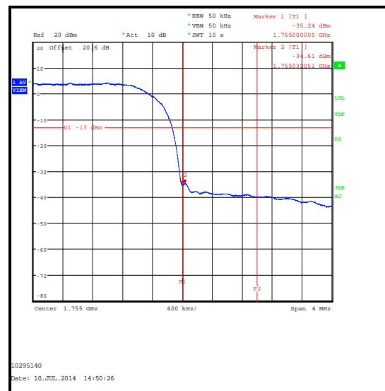
**Transmitter Radiated Emissions at Band Edges (continued)****Results: HSUPA Sub-Test 3**
