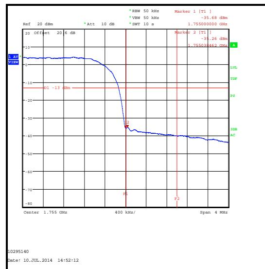
Transmitter Radiated Emissions at Band Edges (continued)Results: HSUPA Sub-Test 2
