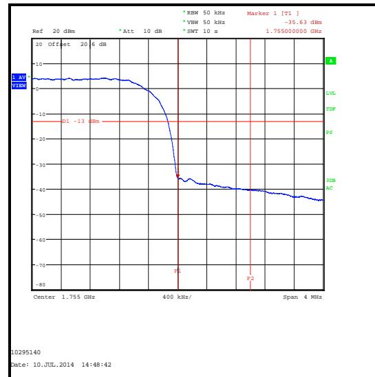
Transmitter Radiated Emissions at Band Edges (continued)Results: HSUPA Sub-Test 4
