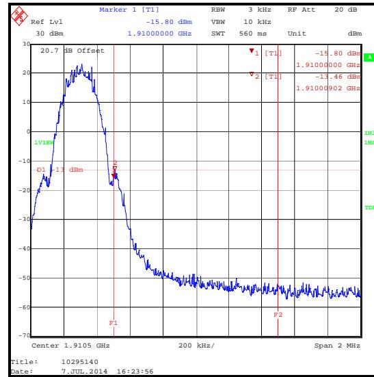
**Transmitter Band Edge Radiated Emissions (continued)****Results: GPRS**
