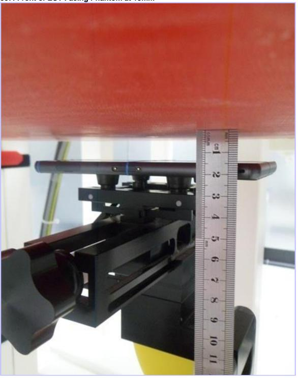
008: Back of EUT Facing Phantom at 10mm
