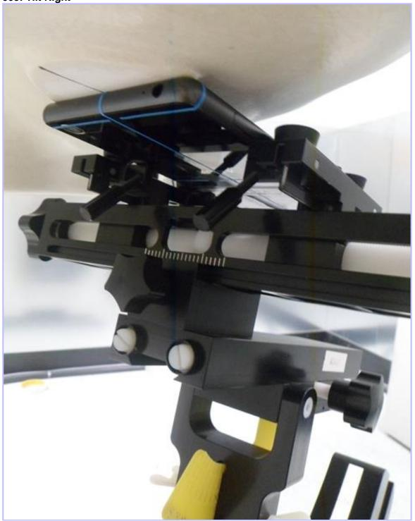
006: Front of EUT Facing Phantom at 10mm
