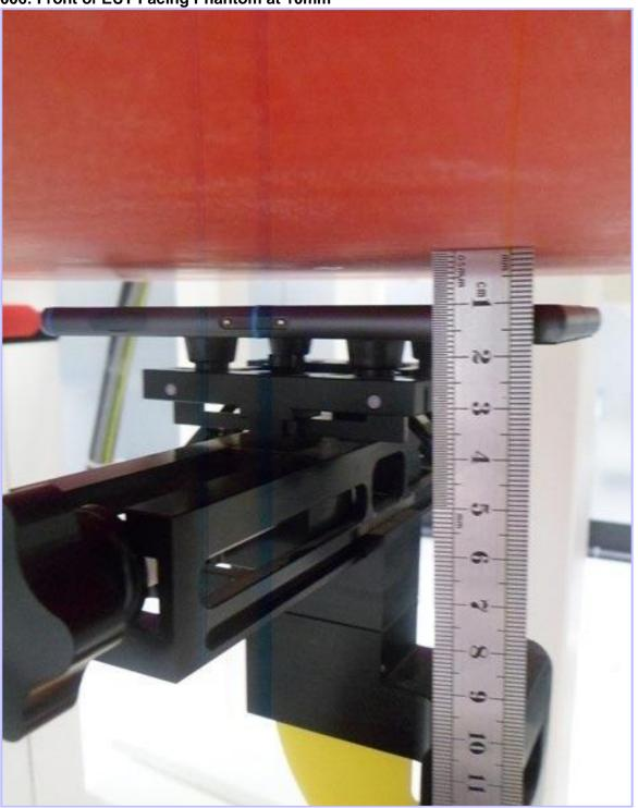
007: Front of EUT Facing Phantom at 15mm
