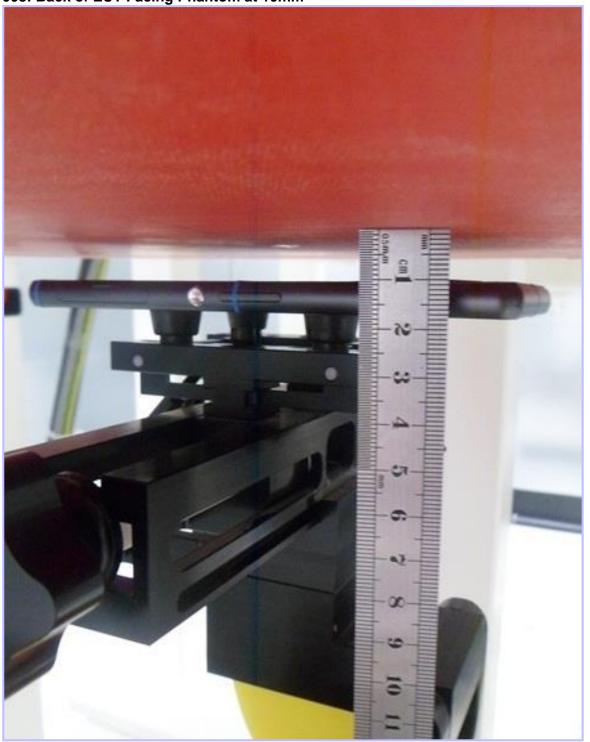
009: Back of EUT Facing Phantom at 15mm
