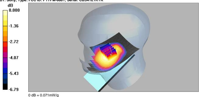
Communication System: LTE - Band 12 / 10MHz Channel; Frequency: 704 MHz; Duty Cycle: 1:1
