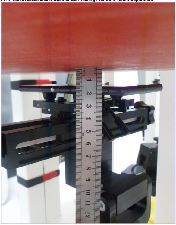
PHT/ 10295122JD06/010: Left Hand Side of EUT Facing Phantom 10mm Separation
