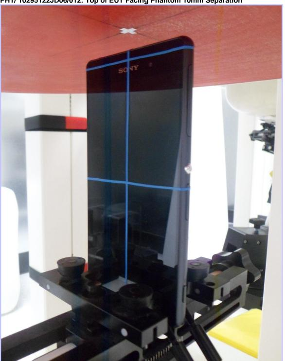
PHT/ 10295122JD06/013: Bottom of EUT Facing Phantom 10mm Separation
