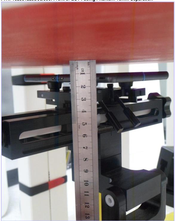
PHT/ 10295122JD06/007: Front of EUT Facing Phantom 15mm Separation
