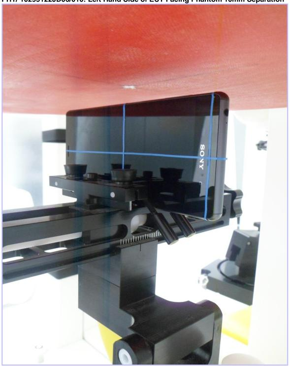
PHT/ 10295122JD06/011: Right Hand Side of EUT Facing Phantom 10mm Separation
