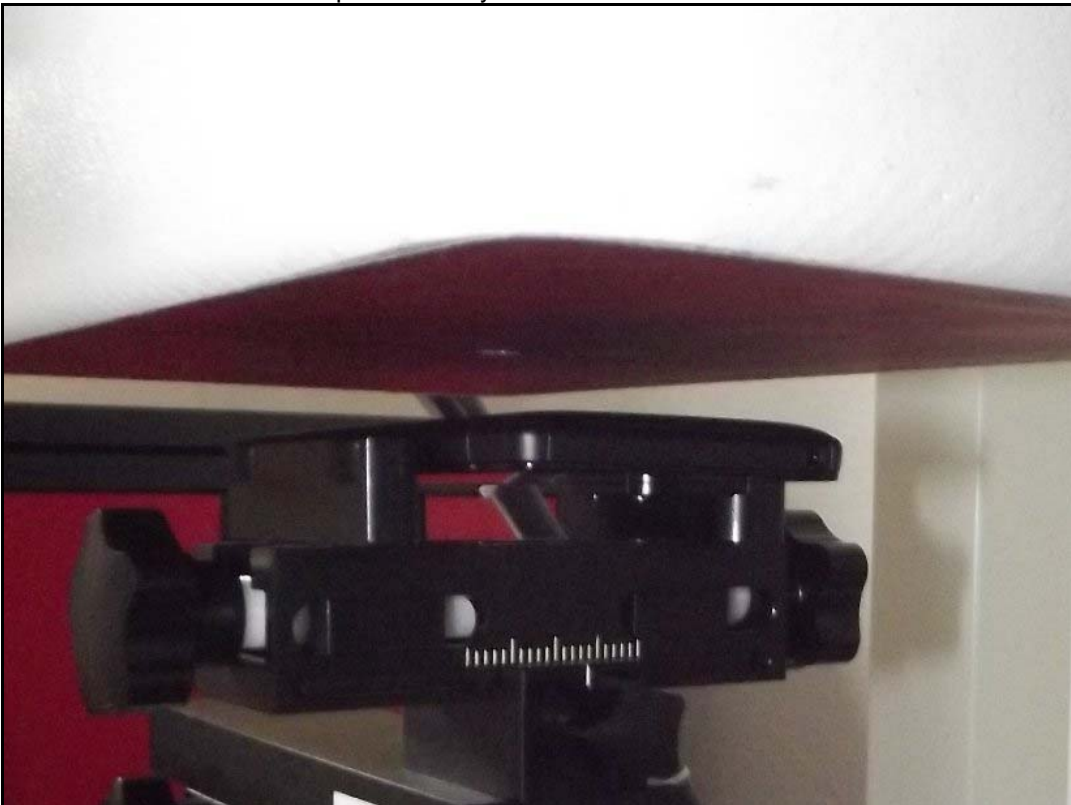
Photo 16: Test position body worn rear side with 15 mm distance
