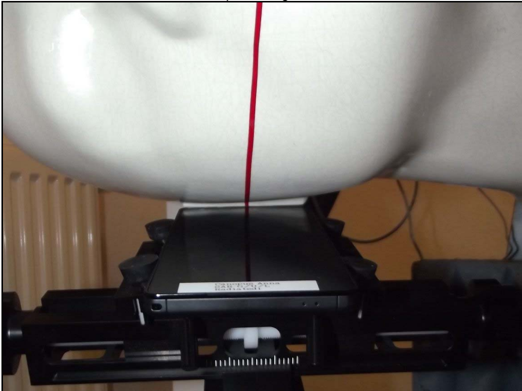
Photo 14: Test position right hand tilted 15°
