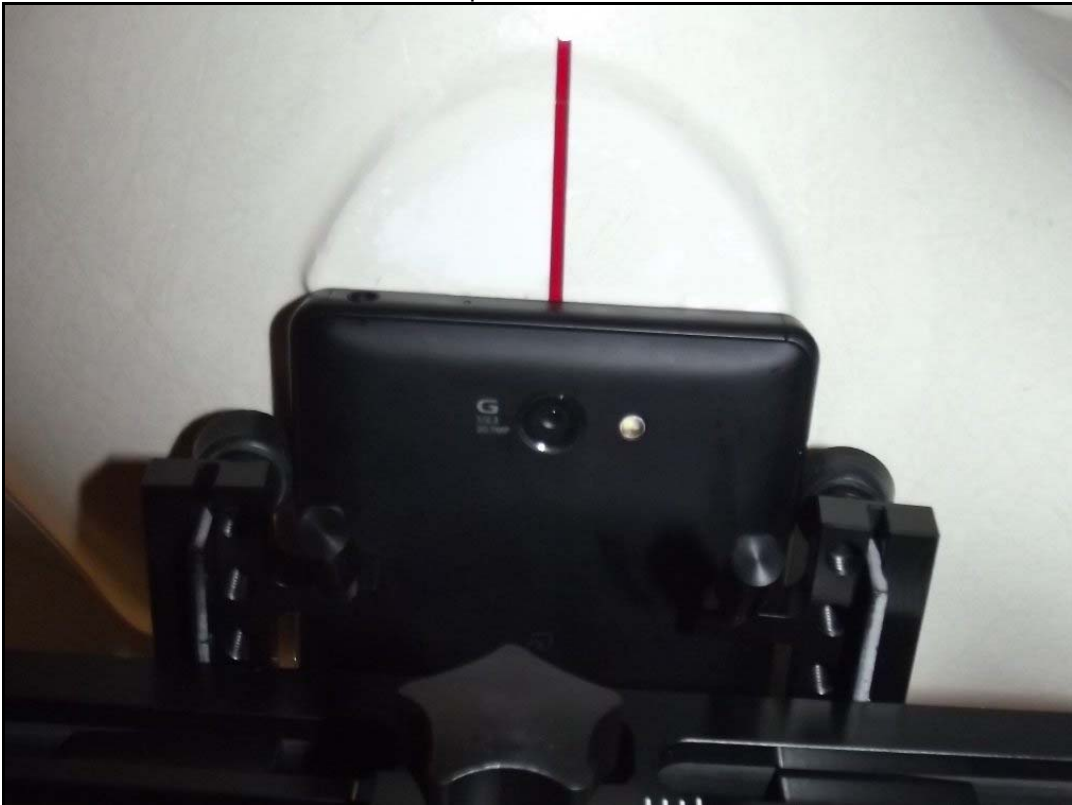
Photo 8: Test position left hand tilted 15°
