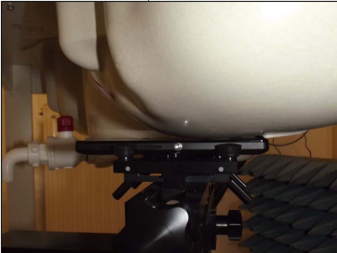
Photo 6: Test position left hand touched
