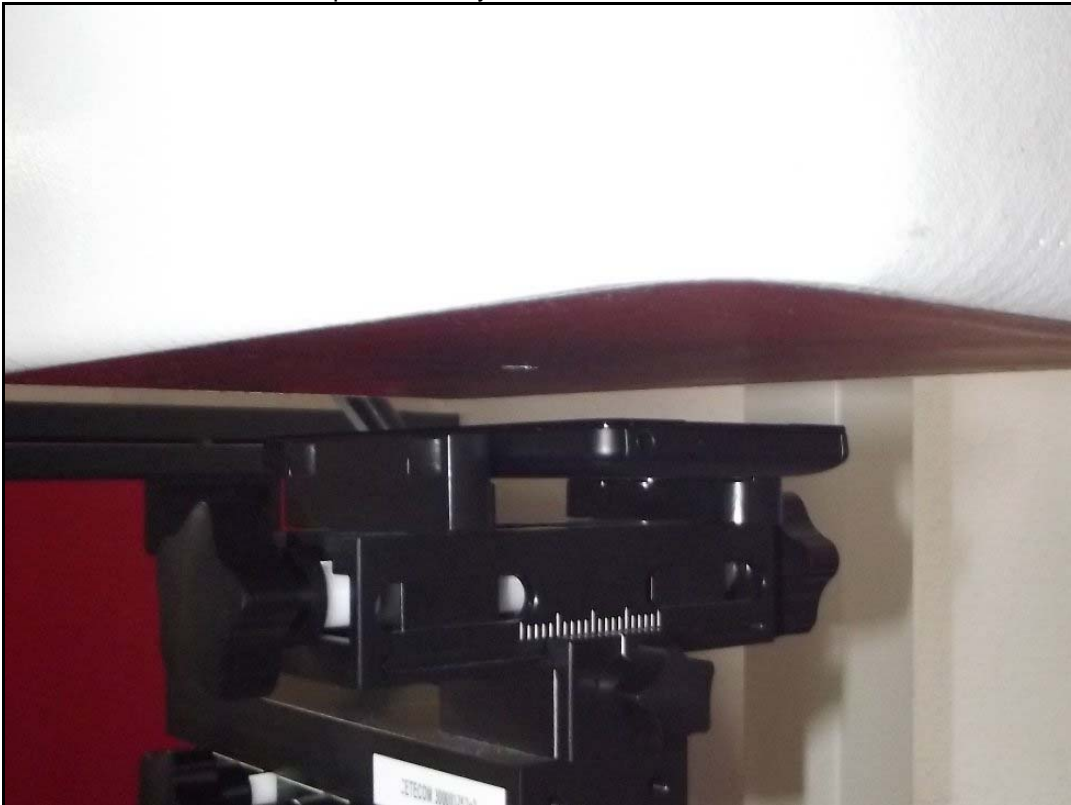
Photo 16: Test position body worn rear side with 15 mm distance
