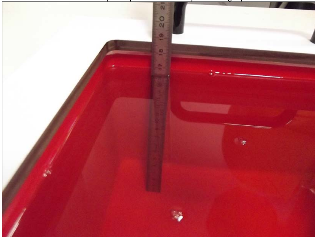
Photo 2: Liquid depth 750 MHz body simulating liquid
