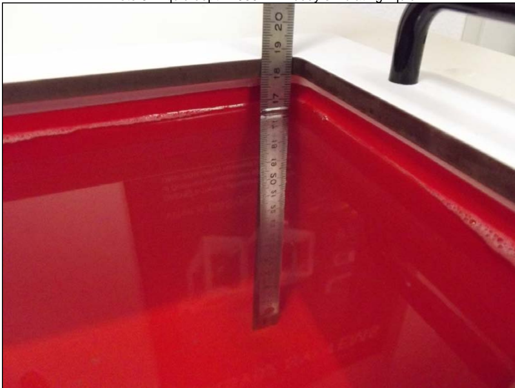
Photo 6: Liquid depth 1900 MHz body simulating liquid
