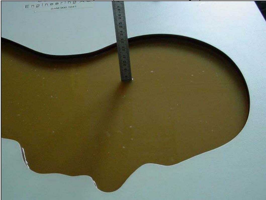
Photo 10: Liquid depth 5 GHz body simulating liquid
