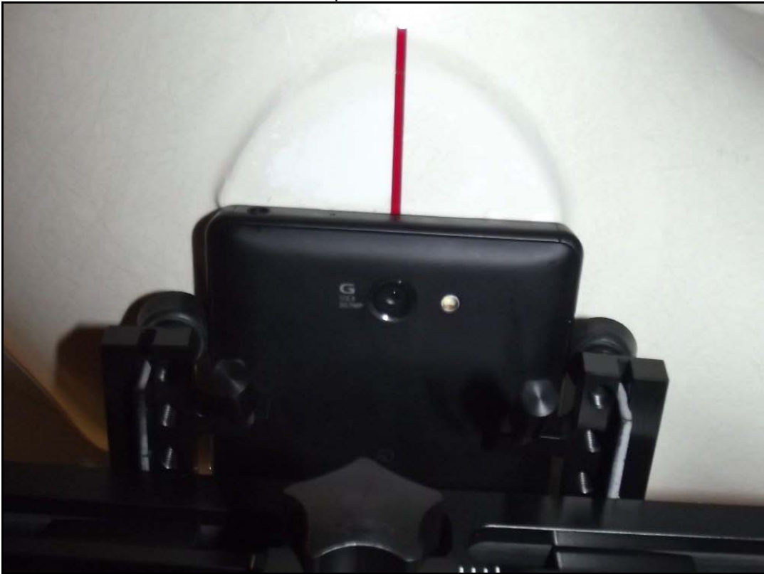
Photo 8: Test position left hand tilted 15°
