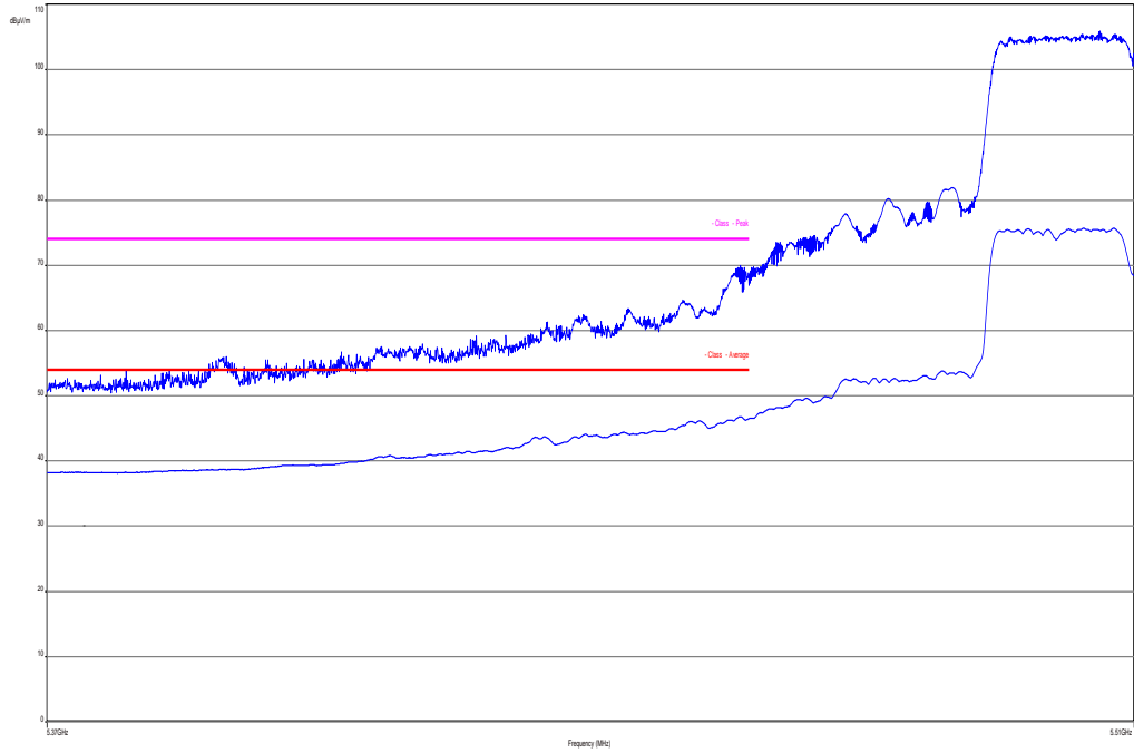
Plot 23: lower band edge, vertical & horizontal polarization (ac HT 40 mode), channel 102, high data rate
