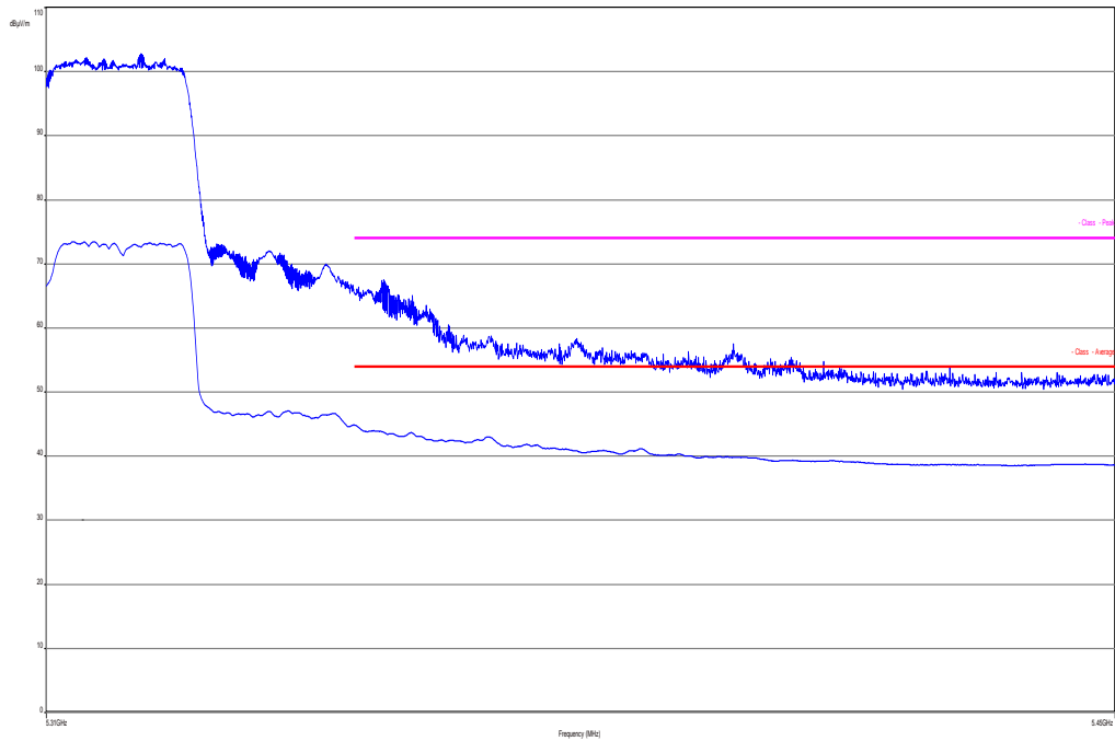
Plot 20: upper band edge, vertical & horizontal polarization (ac HT 40 mode), channel 62, high data rate
