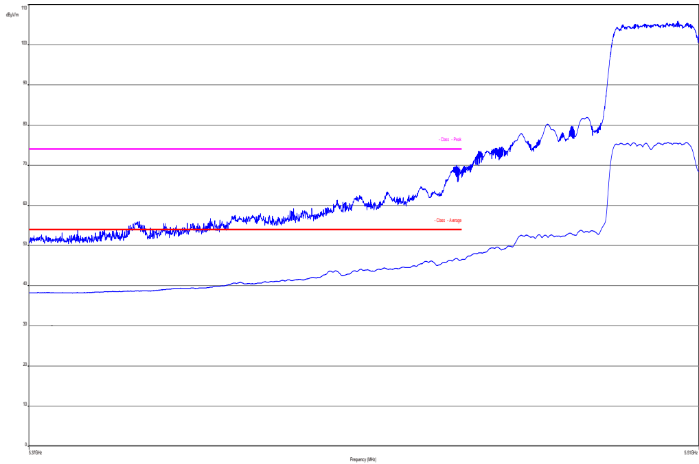
Plot 24: lower band edge, vertical & horizontal polarization (ac HT 40 mode), channel 102, highest power d. r.
