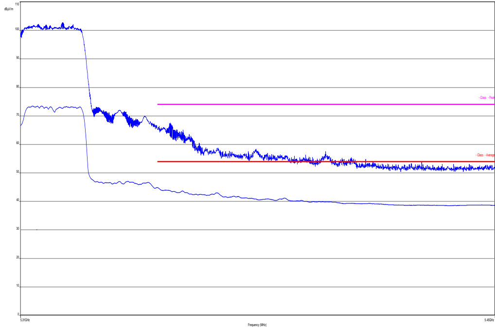
Plot 21: upper band edge, vertical & horizontal polarization (ac HT 40 mode), channel 62, highest power d. r.
