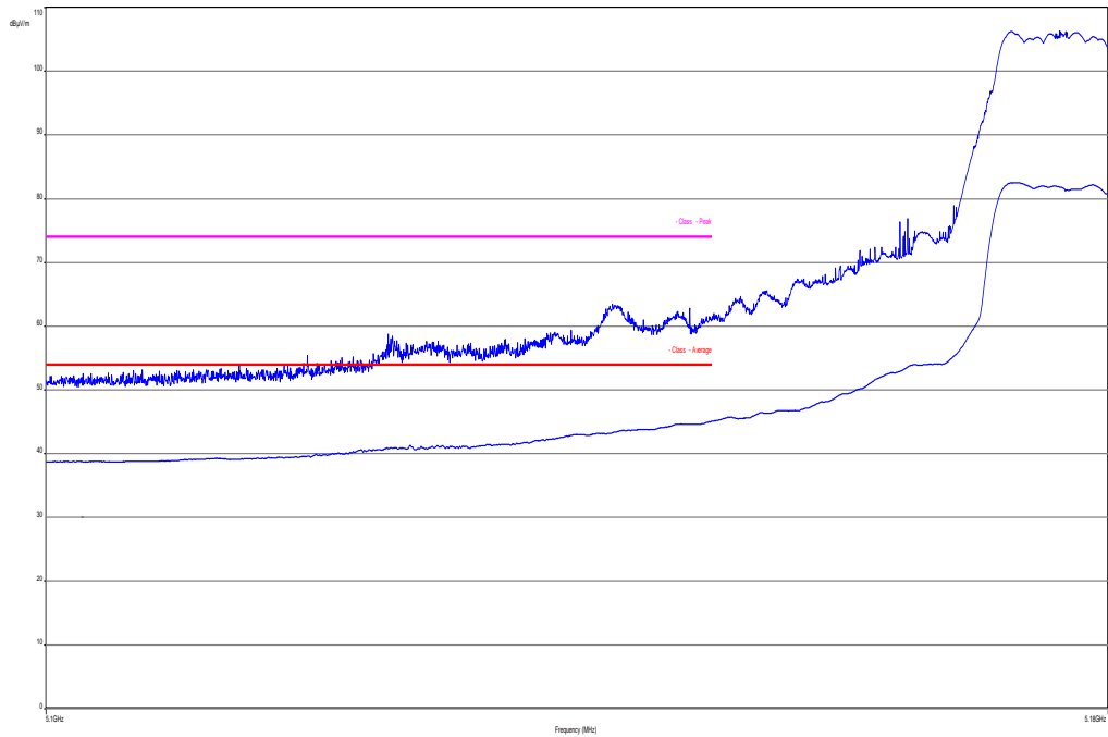
Plot 2: lower band edge, vertical & horizontal polarization (a mode), channel 36, high data rate
