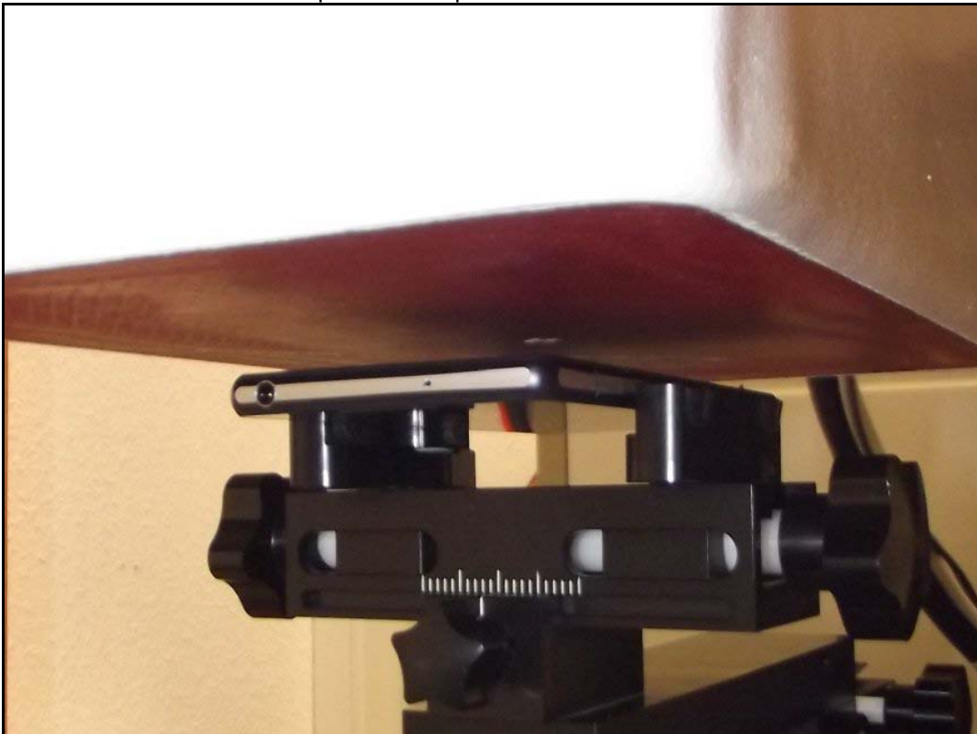
Photo 16: Test position hotspot mode rear side 10mm distance
