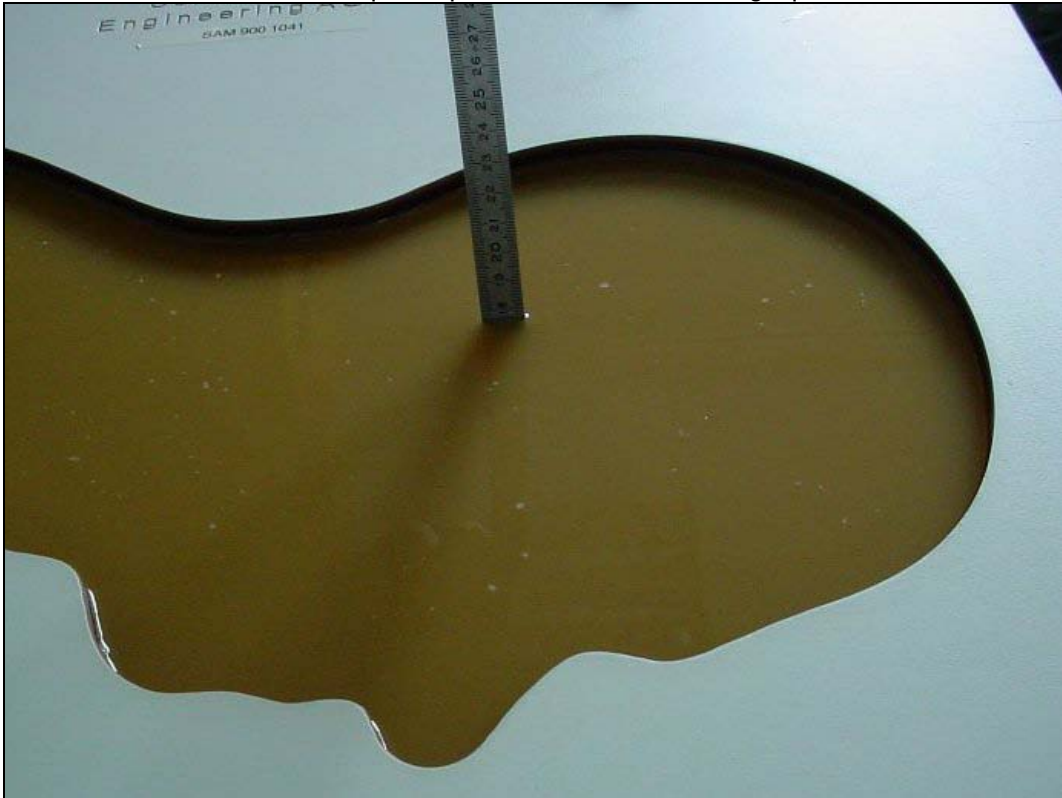
Photo 8: Liquid depth 5 GHz body simulating liquid
