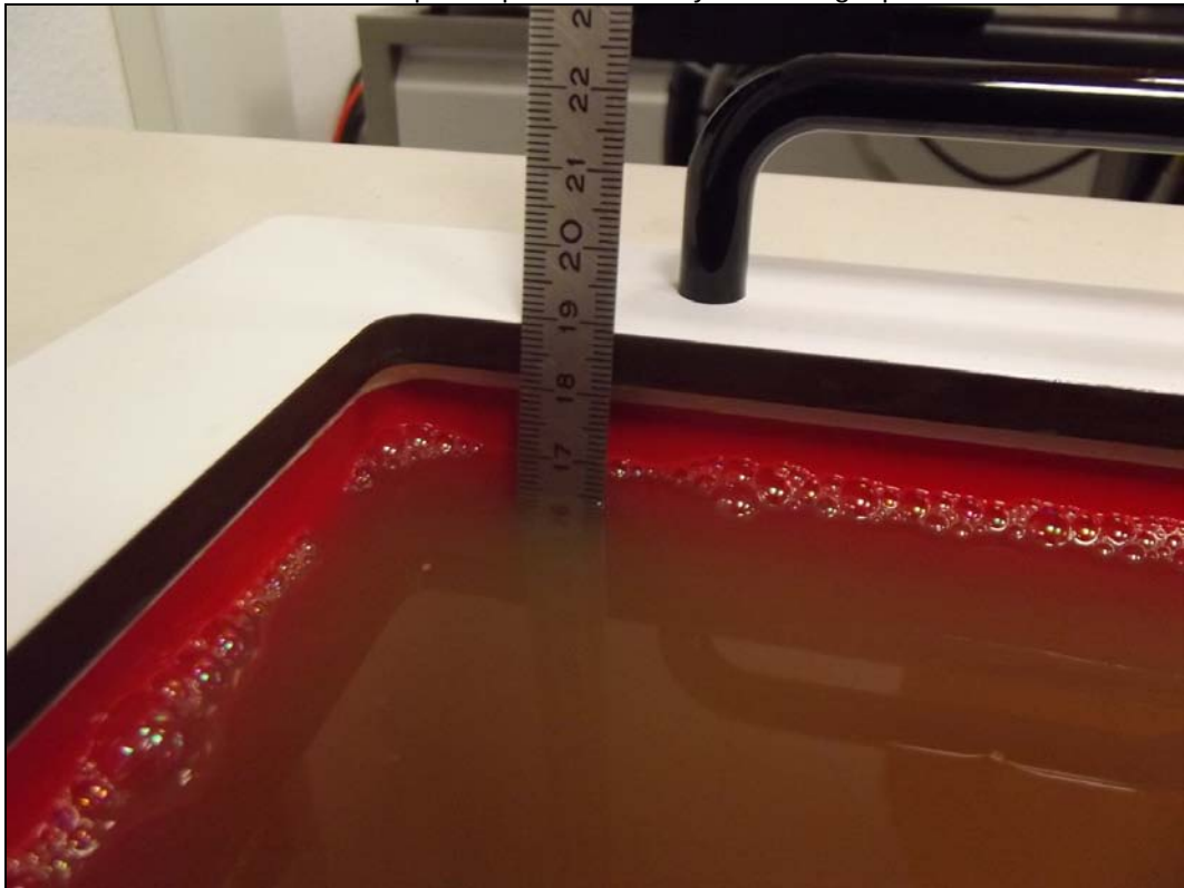
Photo 8: Liquid depth 5 GHz body simulating liquid
