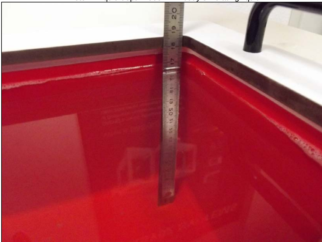
Photo 4: Liquid depth 1900 MHz body simulating liquid
